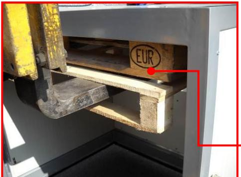
After removing the front door, the unit can be lifted by placing the forks of a lift truck inside the cabinet. Always take care not to damage the inside of the cabinet when lifting it by means of a lift truck.
